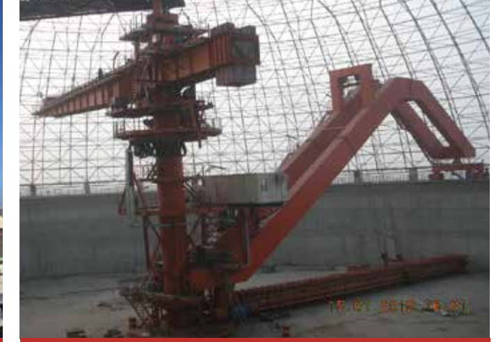
Dairesel Tip İstifleyici Toplayıcı (Yan Tip) Circular Type Stacker And Reclaimer (Side Type)
